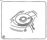
1) Put the bobbin into the bobbin (2) Pull about 4 inches of thread toward you through the tension slot (A).
